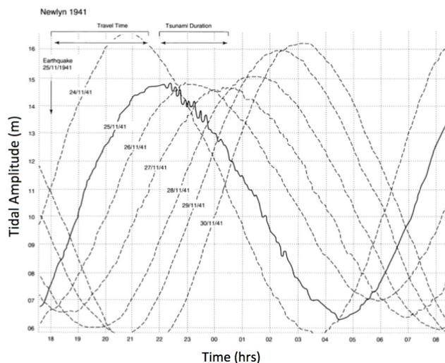
**Fig. 11.** Figure taken from Dawson et al. (2000). Hydrograph showing the arrival of the 1941 Portuguese tsunami at Newlyn, Cornwall (solid line), and the tide gauges on previous and subsequent days (dashed lines) (source: Proudman Oceanographic Institute).
