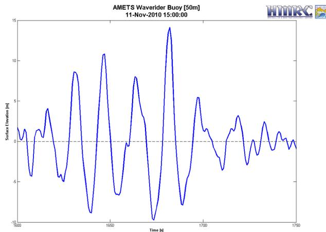
**Fig. 25.** Marine Institute's data for the free surface elevation at the Belmullet wave buoy on 11 November 2010. Retrieved from Brendan Cahill at HMRC, UCC. The time span of the data shown is 150 s. The surface elevation ranges from  $-10$  m to  $+15$  m.
