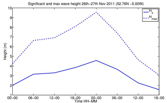
Fig. 23. ECMWF global wave model 6-hourly output of significant and maximum wave heights,  $H_s$  and  $H_{max}$ , respectively, bilinearly interpolated to a location in the region where the *Swanland* sank ( $52.76^\circ$  N,  $-5.00^\circ$  W) on 26–27 November 2011.
