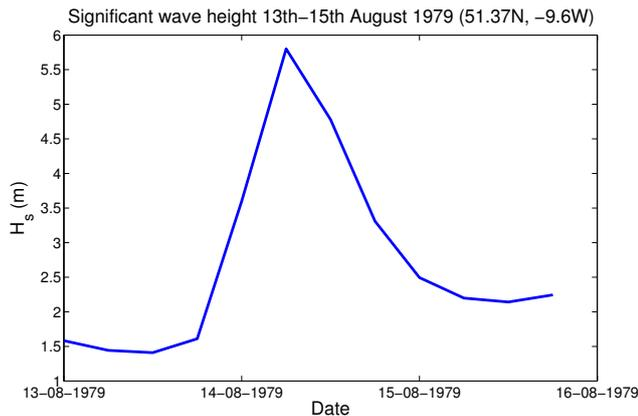
**Fig. 7.** ECMWF model data every 6 h from ERA-Interim reanalysis: significant wave height in the Irish Sea ( $51.37^{\circ}$  N,  $-9.6^{\circ}$  W) during the Fastnet Race 1979 disaster, 13–15 August.
