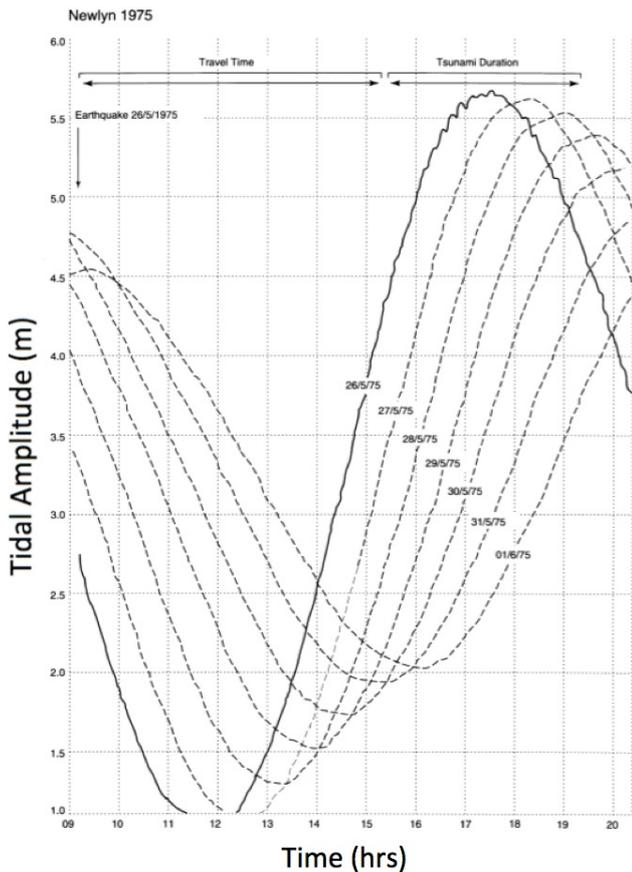
Fig. 12. Figure taken from Dawson et al. (2000). Hydrograph showing the arrival of the 1975 Portuguese tsunami at Newlyn, Cornwall (solid line), and the tide gauges on subsequent days (dashed lines) (source: Proudman Oceanographic Institute).
