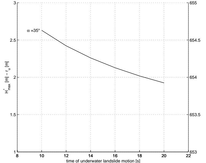
**Fig. 9.** Estimated maximum wave height  $H_{\max}$  generated by the landslide event of 4 November 1960 occurred at the Vajont reservoir. The secondary y-axis refers to levels above the m.s.l.
