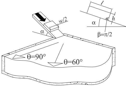
**Fig. 1.** Sketch of the experiment on the study of landslide generated impulse waves propagating in a three dimensional water body.
