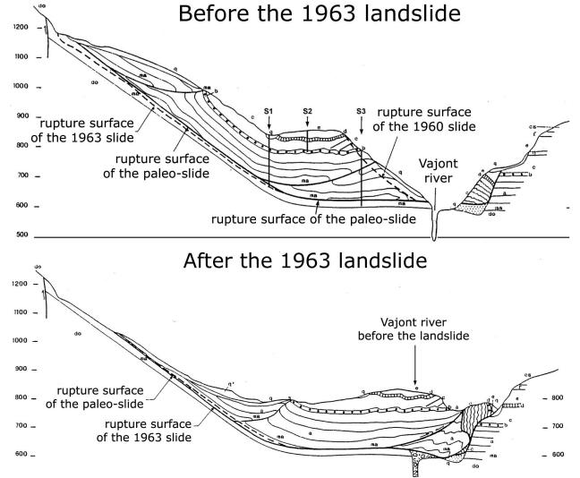
**Fig. 8.** Sections of the Vajont valley before and after 9 October 1963, landslide. The presence of paleo-slide at the Toc mountain is visible in both the panels, presenting a rupture surface very close to the rupture surface of the 1963 slide. A section of the landslide occurred in 1960 is also visible in the left panel (picture taken from Semenza, 2002).
